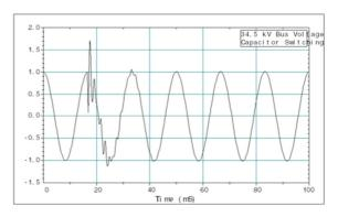
caused by capacitor switching, and high-frequency transients with frequency components in the few-hundred-kilohertz region typically caused by lightning and inductive loads. Transients not only can cause equipment to malfunction and fail: they can also cause insulation to break down, leading to premature failures transformers.
