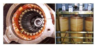
When a transient reaches the coil of a motor or a transformer it will dissipate the majority of its energy in the first few coils. Each successive coil presents more resistance and capacitance to the transient. This will reduce its magnitude and increase its period, reducing the energy. Since the majority of the energy is transferred to the first few coils, this is where the damaged insulation will typically appear.
