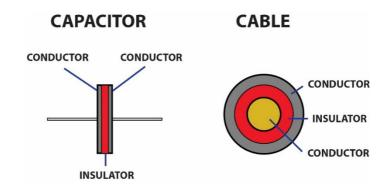
Both capacitors and wires have two conductors separated by an insulator.
