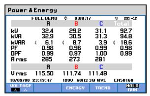
**Figure 3.** By selecting "Power and Energy" from the main menu the Displacement Power Factor (DPF) can be observed to ensure specifications for power supplied to the VFD are met. Use DPF unless the manufacturer specifies power factor is to take into account harmonic frequencies, then use the PF reading. Note the inductive coil symbol in the kVAR line indicates the current power factor is lagging.
