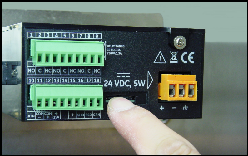
Figure 53: Pushing in on the MicroSD Card
