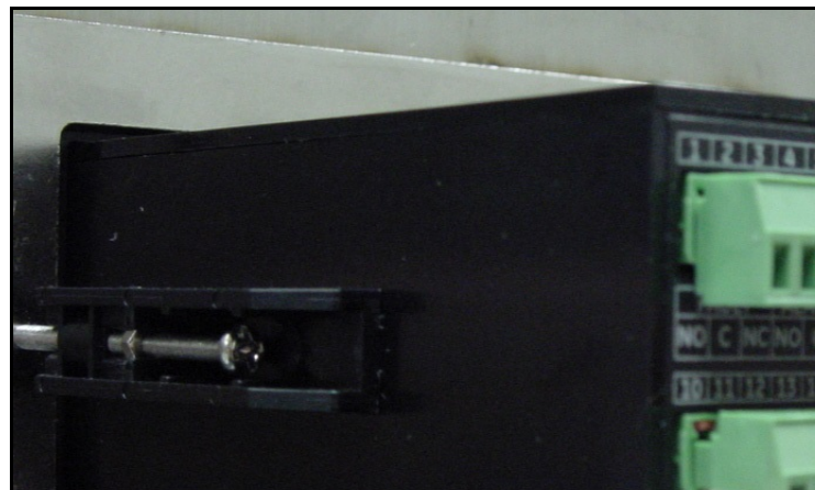
Figure 36: Reinserting the Connector into the Terminal Block
