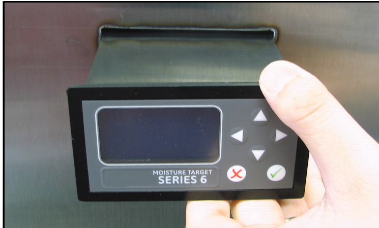
Figure 11: Sliding the MTS6 into the Panel Cutout
