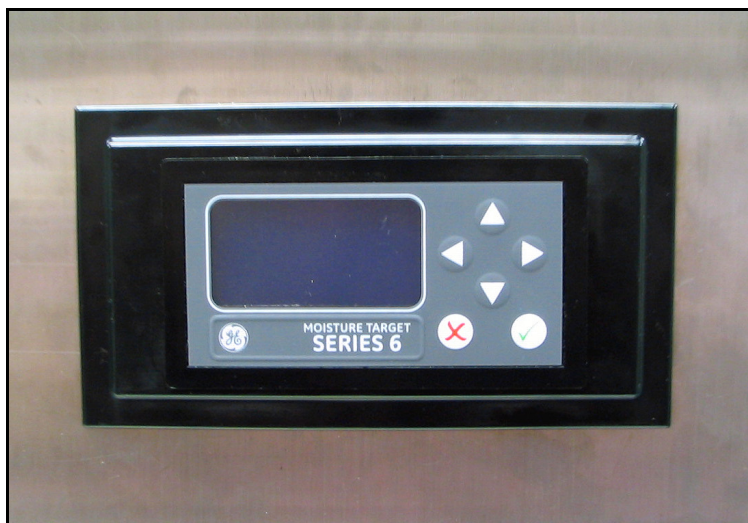
Figure 22: MTS6 Installation with Adapter Plate – Front
