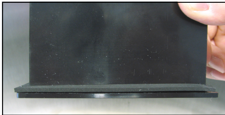
Figure 10: Installing the Gasket Behind the Display
