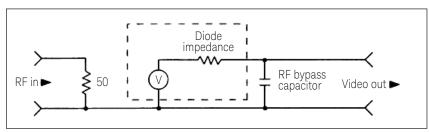
Figure 7. Detector equivalent circuit
