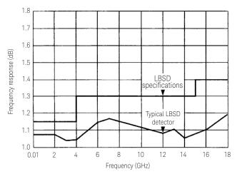
Figure 3. Detector SWR specifications
