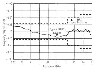
Figure 2. Detector frequency response specifications
