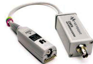
Horizontal and vertical versions of the PC board mini-probe socket make it easy to fit into your target board.
