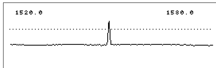
PRBS modulation graph showing raised noise floor.
