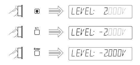
Channel 1's trigger level is now set to -2V.
