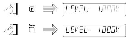
Channel 1's trigger level is now set to +1V.
