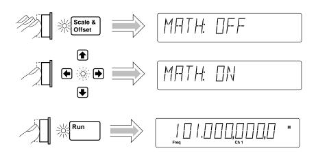
The result of this Math operation is a measurement of 101 MHz.
