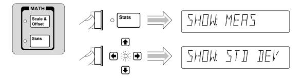
Updating the SHOW configuration caused Stats to be enabled. The Stats indicator is now lit.
