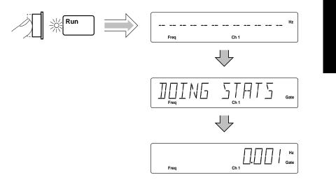
The Counter is now set to make statistics based on 20 measurements.
