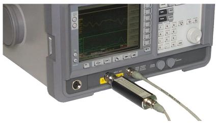
Figure 4-4 Operator's check test setup 2b
