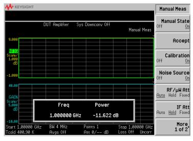
Figure 4-5 Typical example of power reading with Noise Source On
