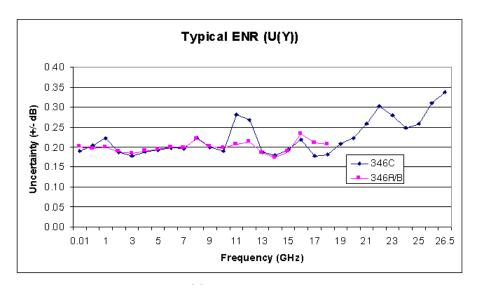
Figure 3-1 Characteristic<sup>[1]</sup> ENR plot versus cardinal frequency points
