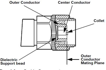
Figure A-1 Precision 7 mm connector
