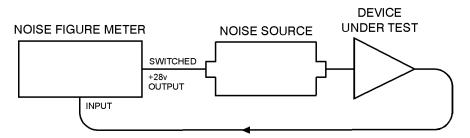
Figure 4-1 Typical noise figure measurement test setup
