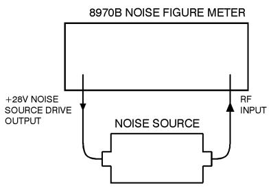
Figure 4-3 Operator's check test setup 2a
