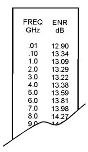
Figure 1-1 A partial view of typical calibration label
