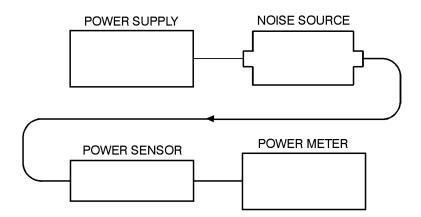
Figure 4-2 Operator's check test setup 1
