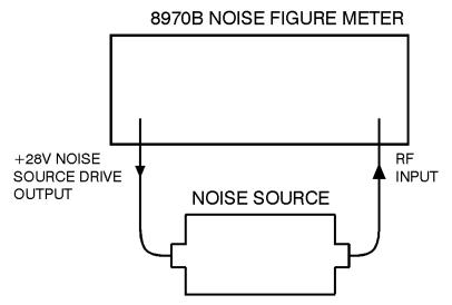
Figure 4-3 Operator's check test setup 2a
