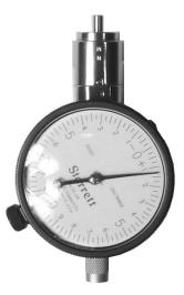
Figure A-6 Using the connector gage
