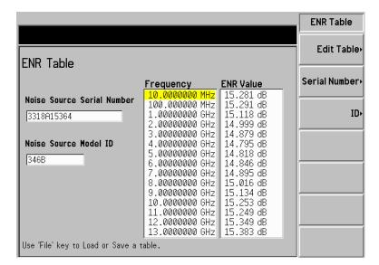
Confirm that the noise source Serial Number and the noise source Model ID are correct, and compare the Frequency and ENR values with the supplied Calibration Sheet or the data printed on the body of the noise source.
