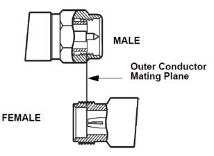
Figure A-2 Precision 3.5 mm connectors
