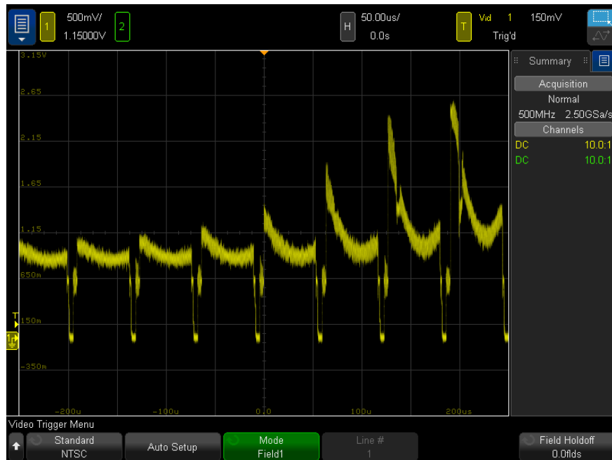
Figure 22 Triggering on Field 1
