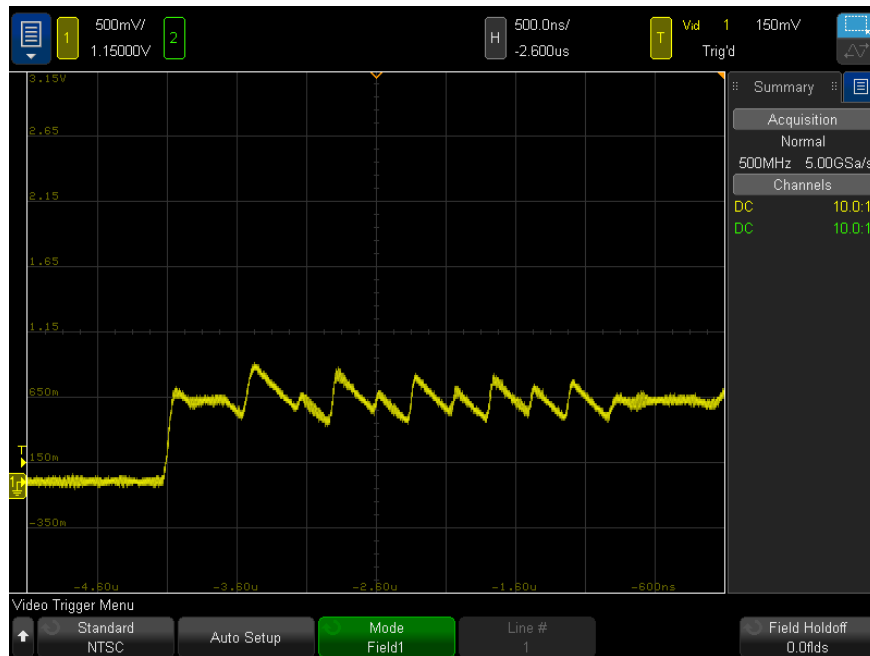
Figure 24 Triggering on Color Field 1 Alternating with Color Field 3
