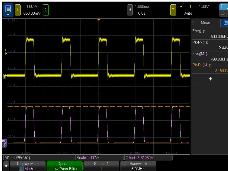
Figure 15 Example of Low Pass Filter
