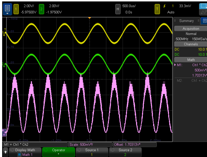
Figure 5 Example of Multiply Channel 1 by Channel 2
