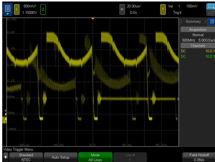
Figure 21 Triggering on All Lines
