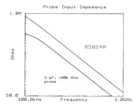
Probe with less error due to higher input impedance. For example, in a 50  $\Omega$  system at 500 MHz, the 85024A presents 455  $\Omega$  which produces a 10% signal loss from loading effects, while a 3 pF, 100 k $\Omega$  probe presents 106  $\Omega$  causing a 32% signal loss.
