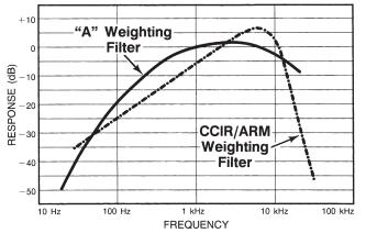
CCIR/ARM Weighting Filter (CCIR rec. 468-2, averageresponding meter, Dolby Labs Bulletin No. 19/4)
