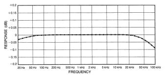
Typical flatness of source and analyzer combined (source voltage set to 1 V, 1 kHz reference).
