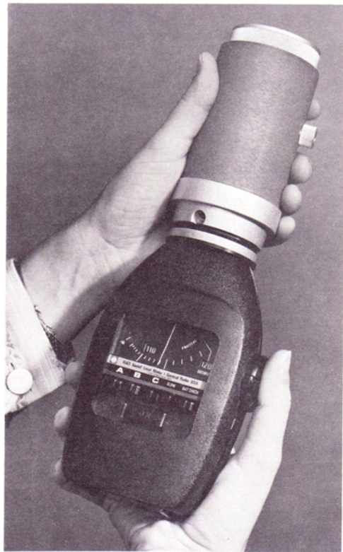
Figure 4. Type 1567 in use calibrating a sound level meter.
