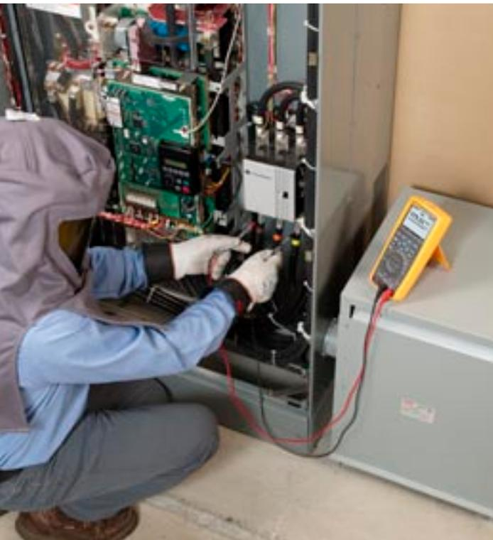
has been reached, then it beeps and freezes (holds) a stable reading on the display for the user to see. If the input changes to the point that it is no longer stable, then becomes stable again, the meter will beep a second time and hold a new reading on the display.
