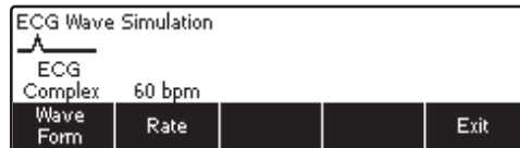
Figure 31. ECG Waveform Simulation Menu
