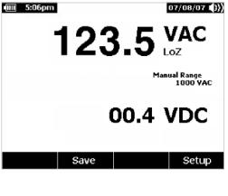
such as in the same conduit or raceway. This condition forms a capacitor and allows capacitive coupling between the energized wiring and the adjacent unused wiring.
