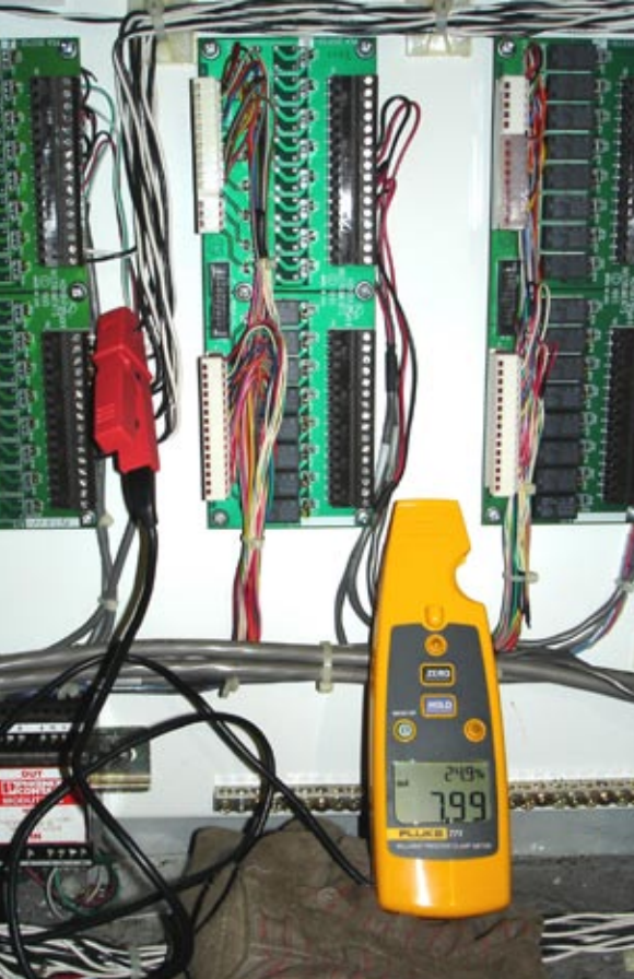
Figure 2: In specific applications, percentage readings on the Fluke 771 may be more useful than the underlying current readings – for example, when a control output must be maintained within a range of 25-30 % of the maximum level. Here, the Fluke 771 is connected to the emission control loop.
