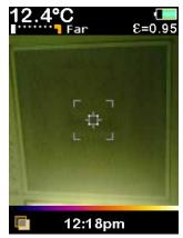
Use your visual IR thermometer to see how well the VAV box is working by scanning vents. The warm area in this otherwise cold vent could indicate a faulty cold air damper.
