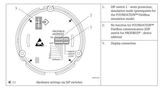
The simulation mode via the hardware setting has priority over the software setting.
