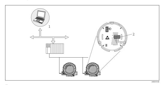
1 Configuration∕operating programs for operation via FOUNDATION Fieldbus™ (Foundation Fieldbus functions, device parameter)
