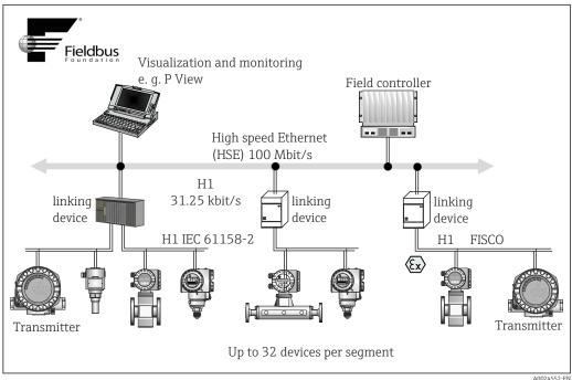
System integration via FOUNDATION Fieldbus™
