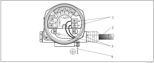
**№** 6 Connecting the device to the FOUNDATION Fieldbus fieldbus cable
