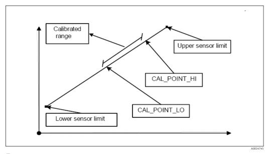
■ 21 Linear scaling of temperature-linear curve
