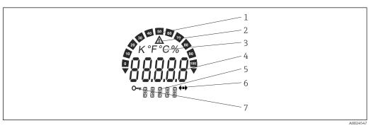
■ 10 LC display of the field transmitter (illuminated, can be plugged in in 90° steps)
