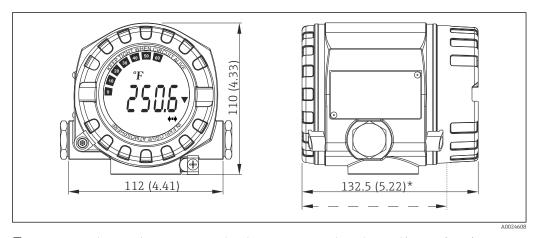
ightharpoonup 17 Die-cast aluminum housing for general applications, or optional stainless steel housing (316L)
