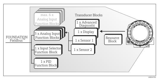
■ 19 Block model of the temperature field transmitter
