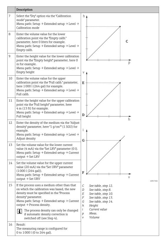
For this level mode, the measured variables %, level, volume and mass are available, see "Unit before lin." .
