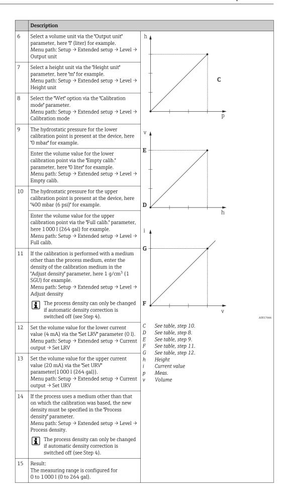
The measured variables %, level, volume and mass are available for this level mode, see "Output unit".
