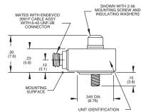
STANDARD TOLERANCE INCHES (MILLIMETERS) .XX = +/- .02 (.X = +/- .5)
