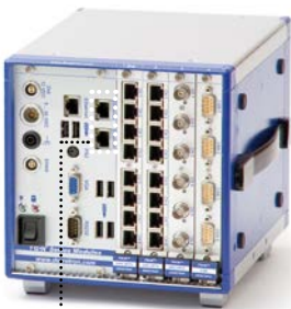
DW2-LAN-2 DEWE2-M4s with 2x 1 Gbit Ethernet option
