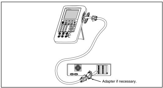
Figure B-1. Connecting the Calibrator
