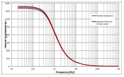
Figure A20. Transfer Impedance vs. Frequency.
