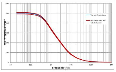
Figure A8. Transfer Impedance vs. Frequency.
