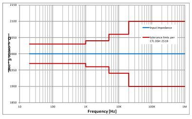
**Tolerance comparison for LCB Configuration 5**
