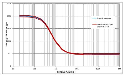
**Tolerance comparison for LCB Configuration 3**
