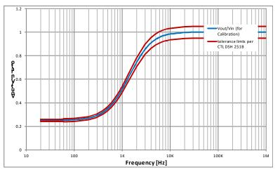
Figure A3. Vout/Vin Ratio vs. Frequency.
