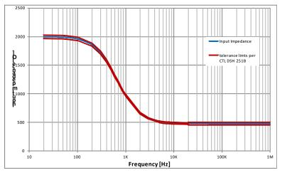
**Tolerance comparison for LCB Configuration 2**
