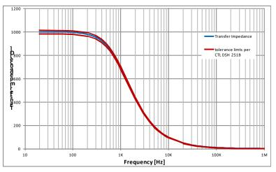
Figure A11. Transfer Impedance vs. Frequency.
