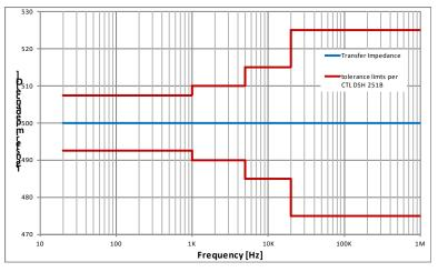
Figure A17. Transfer Impedance vs. Frequency.
