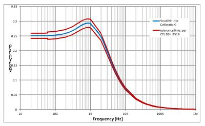
Figure A6. Vout/Vin Ratio vs. Frequency.
