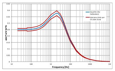
Figure A9. Vout/Vin Ratio vs. Frequency.
