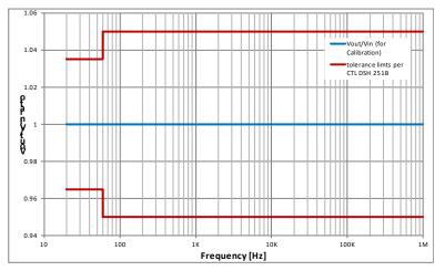
Figure A15. Vout/Vin Ratio vs. Frequency.
