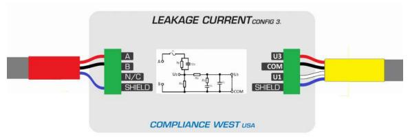
Figure 1: Test lead wiring. Note: if the YELLOW-marked cable for voltmeter connection has only two connections, then only the red and black wires are used (white wire is not used).
