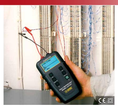
The Fault Mapper Pro® is a hand-held graphical TDR (Time Domain Reflectometer) designed for identifying and locating faults on power and communication cables, given access to one end only.
