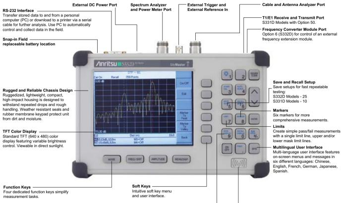
Save and Recall Display Up to 300 memory locations. Alphanumeric data labeling and automatic time/date stamp simplify data management. AM/FM Receiver with Internal Speaker
