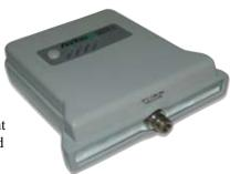
The Site Master S332D integrated Spectrum Analysis capability provides the "ultimate" in measurement flexibility for field environments and applications requiring mobility. With the S332D you can locate, identify, record and solve communication systems problems quickly and easily, and with incredible accuracy – making it a perfect solution for conducting field measurements in the 100 kHz to 3 GHz frequency range.
