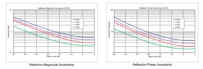
Using the 560-7N50B detector, the following curves show estimated power monitor uncertainties for various DUT match.
