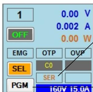
This tile represents a group of series-connected channels. Voltage and power readings show the total value for the group.
