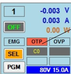
The PV simulator power stage overheated and the output has been turned off. Wait until the unit cools down and the output is restored. This should never occur, even on hot days and full power operation and it is an indication of a hardware malfunction.
