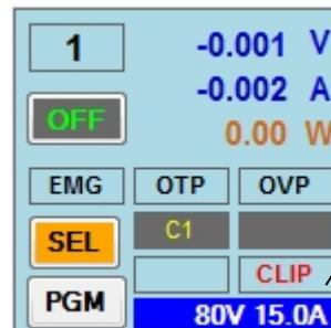
The assigned curve or array, translated to the programmed irradiance and temperature, exceeded the maximum voltage or current capability of the channel. The curve has been clipped to fit into the channel's voltage and current ratings.
