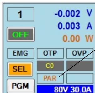
This tile represents a group of parallel-connected channels. Current and power readings show the total value for the group.
