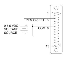
Figure 3-17. Remote Overvoltage Programming Using DC Source
