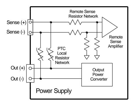
Figure 3-22. Remote Voltage Sensing Network
