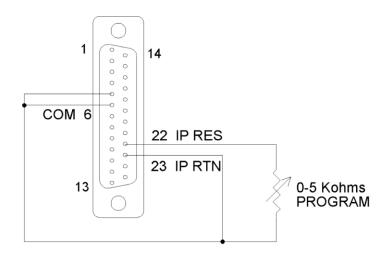
Figure 3-13. Remote Current Programming Using Resistance
