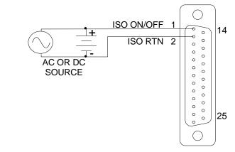
Figure 3-19. Remote Isolated Output ON/OFF Using AC or DC Source
