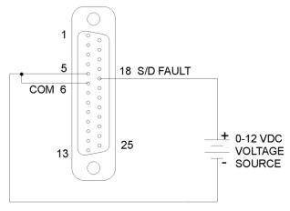
Figure 3-21. Remote Shutdown Using DC Voltage Source
