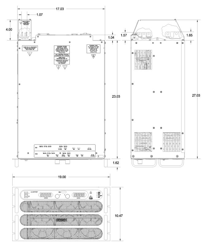
Figure 2-5. Installation Drawing, 6U Models 20 kW to 30 kW
