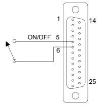
Figure 3-18. Remote Output ON/OFF Control by Contact Closure
