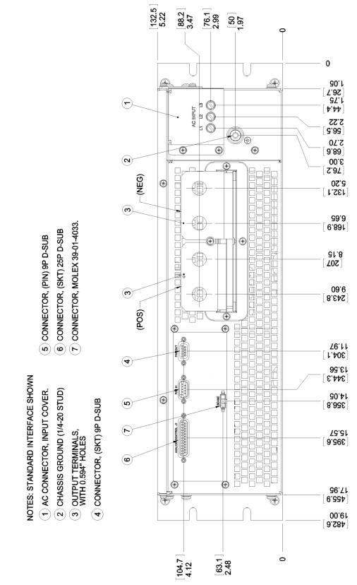
Figure 2-6. Rear Panel, Standard, 3U Models 10V-30V
