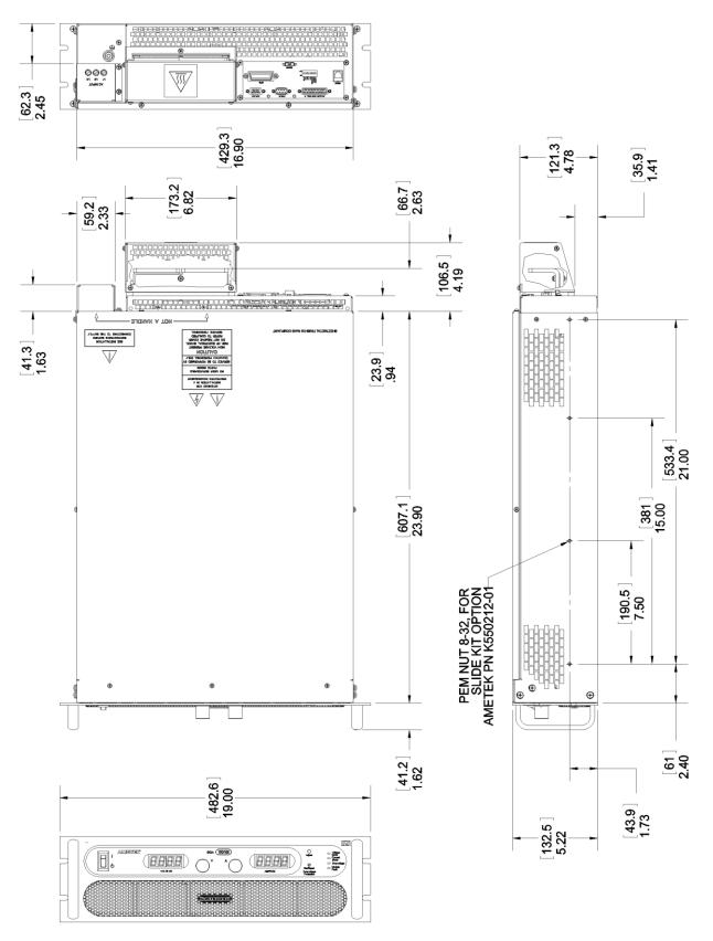
Figure 2-2. Installation Drawing, 3U Models 10V-30V
