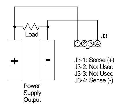
Figure 3-24. Remote Sense Connection at the Load, 1000V Model
