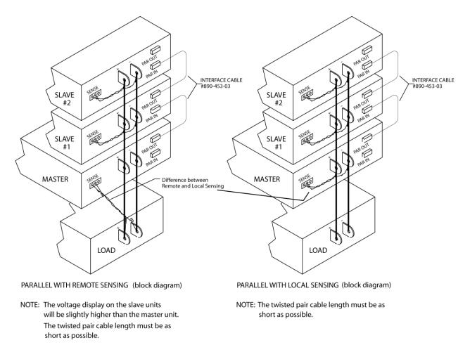
Figure 3-25. Parallel Connection and Remote Sense
