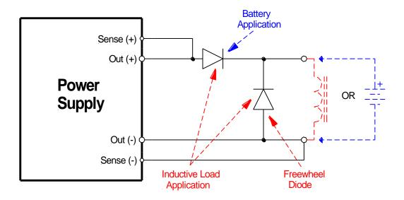
Figure 2-1. Diode Connection
