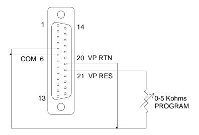
Figure 3-15. Remote Voltage Programming Using Resistance
