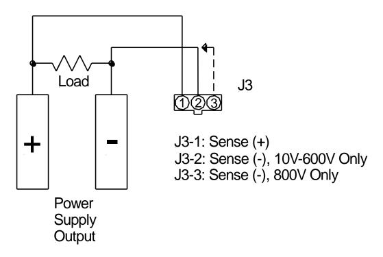
Figure 3-23. Remote Sense Connection at the Load, 10V-800V Models
