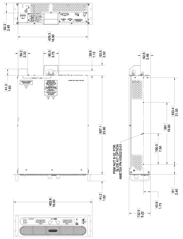
Figure 2-4. Installation Drawing, 3U Models 800V-1000V
