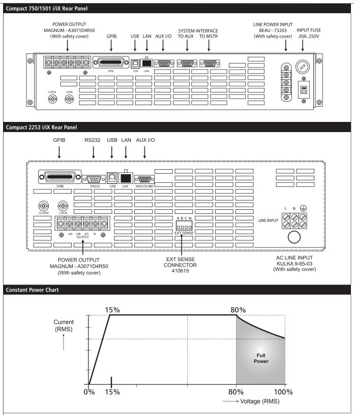
Note: Constant power mode provides increased current at reduced voltage. Maximum available current shown.
