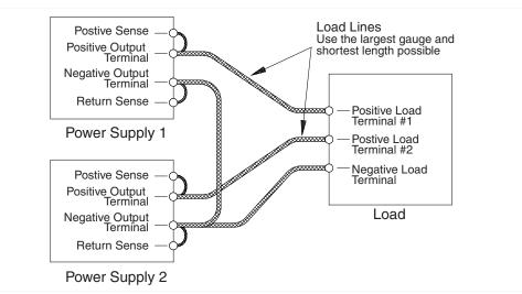
Figure 4.4 Split Supply Operation of Multiple Supplies (two positive voltages)
