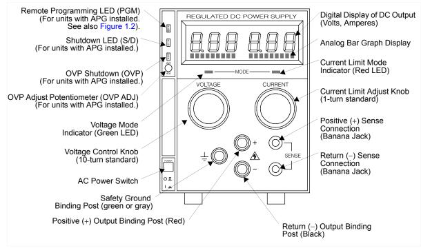
Figure 1.1 Front Panel Controls
