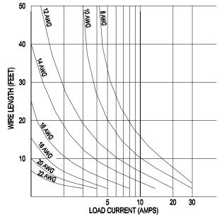
Figure 3.1 Maximum Wire Length for 100 mV Line Drop
