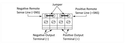
Figure 3.2 Output Barrier Strip With Jumpers Installed
