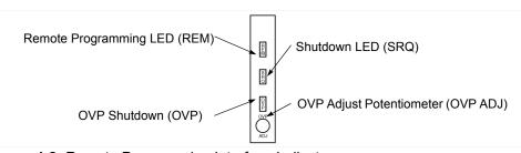
Figure 1.2 shows the programming interface indicators for units that have a digital programming interface installed.
