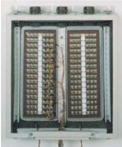
View of a 64-channel UTR. Kaye has also supplied custom UTR's, such as 64-channel units, some with special connectors and water cooling tubes. Custom UTR's have been developed for Rolls-Royce, Arnold Air Force Base, General Electric and Pratt & Whitney.
