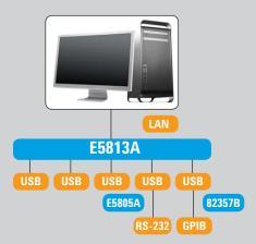
You will obtain the best performance when you do the fewest format conversions. For example, using the E5810A (LAN to GPIB), data transfer will generally be faster than 82357B and an E5813A (LAN to USB to GPIB).
