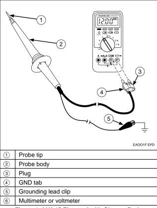
Figure 1. 80K-15 Electronic Air Cleaner Probe
