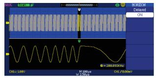
Use the oscilloscope's delayed sweep feature to zoom in a particular area of a signal in real time while viewing the entire captured waveform simultaneously.
