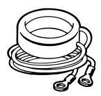
A Donut Current Transformer enables this meter to monitor motors with current ratings up to 1000 amps. The Donut (also known as a "Toroid") is placed around one of the legs of the device being monitored, and emits up to a 5 amp signal. Each Donut Transformer, rated at 2 volt amps, comes with 2' long secondary leads.
