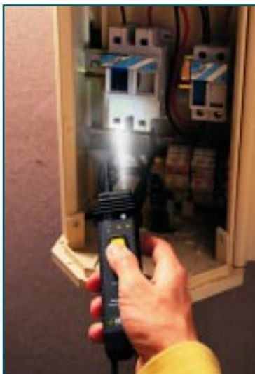
Remote Test Probe used with Models 1050 or 1060 with target light activated
