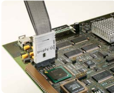
E5346A 34-channel Mictor connector probe
