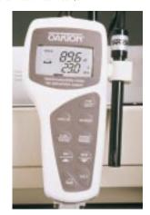
ready to import into spreadsheet applications. Switch from conductivity to TDS readings with one button press. Calibrate up to 5 Conductivity or TDS calibration points. Stores and recalls up to 16 sets of measurements. Hold function; Auto-Off; Ready indicator. Conductivity/temperature cell included.
