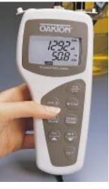
The OAKTON microprocessor-based CON 100 Conductivity/°C meter reads conductivity from 0 to 199.9 mS across five ranges. Display conductivity and temperature simultaneously. Store up to five calibration points. Features include Hold function, Auto-Off option, and Ready indicator.
