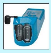
The pH/ORP sensor chamber provides protection to a unique porous liquid-junction.
