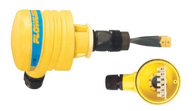
Intended for side wall installation, the general purpose level switch package provides reliable liquid level detection with one 1A relay and a compact junction box for integral wiring termination. Available in two level sensor technologies, select the type and material based upon your application media. This liquid level switch package is widely applied in bulk storage and process tank level applications as a high level alarm or low level alarm.
