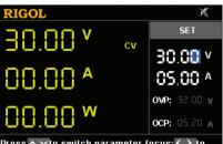
Press ^ / to switch parameter focus; { > to move the cursor;use num key or knob to modify parameter.
