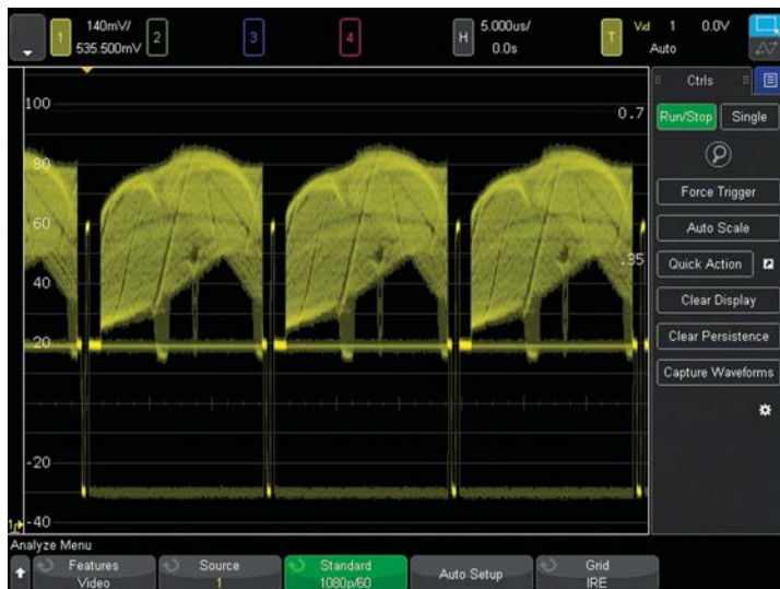
Figure 27. Triggering on 1080p HDTV signal analysis.
