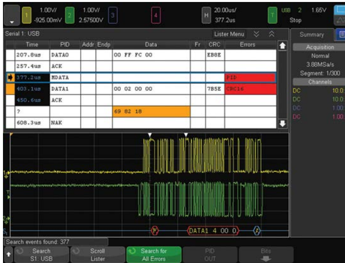
Figure 21. USB 2.0 trigger, decode and "lister" display.
