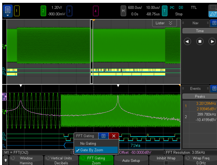
Figure 18. Gated FFT successfully correlated the hopping of the FSK modulation with the analog and I 2 C control command.
