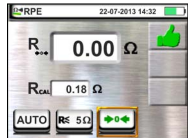
Fig. 7: Compensation of single cables and remote lead resistance
