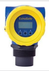
FM approved for hazardous environments, the explosion proof ultrasonic level transmitter provides continuous level measurement up to 32.8' (10m) with a 4-20 mA signal output, and is configured via the integral push button display module. This non-contact liquid level sensor is ideally suited for corrosive, ultrapure, sticky or dirty liquids, and is widely selected for bulk storage, day tank, lift station and process tank level applications located in a classified area.
