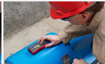
Indicates motor rotation in disconnected motors using test leads and by spinning the shaft by hand or other means.
