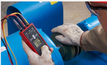
Indicates the phase rotation in 3-phase systems for both power sources and motors.
