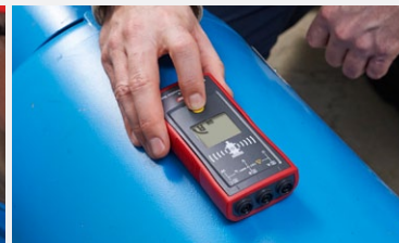
Identifies faulty 3-phase wiring with de-energized phases or incorrectly wired receptacles.
