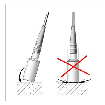
Note: The magnetic transducer should be carefully mounted to the measuring point by "rocking" it into place.
