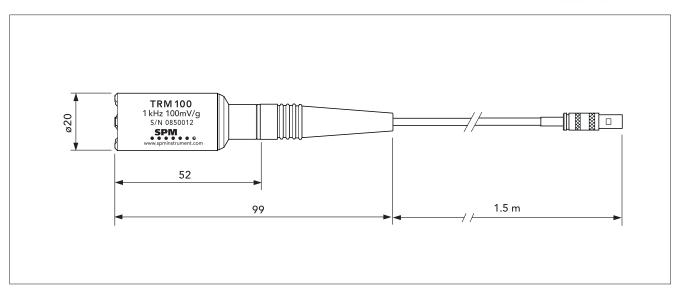
The vibration transducer TRM100 is an accelerometer based on micro-electro-mechanical-systems (MEMS) technologies, designed for vibration monitoring with the handheld instrument SPM VibChecker.
