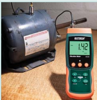
Test vibration levels on motors, bearings, fans, pumps, rotating machinery, and more.
