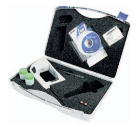
This battery tester offers the ability to test both lead-acid and nickelcadmium batteries with ease. The SBS-2500 offers results within seconds by utilizing the oscillating tube method combined with precise temperature measurement and an elegant user interface. The SBS-2500 gives you reliable measurement results, easily - just immerse the sampling tube, pull the trigger and read the final results.
