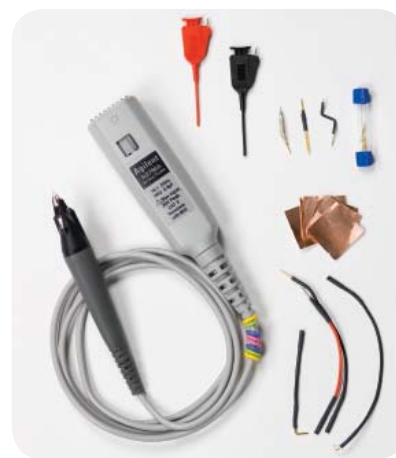
N2795A/96A active probe with standard accessories
