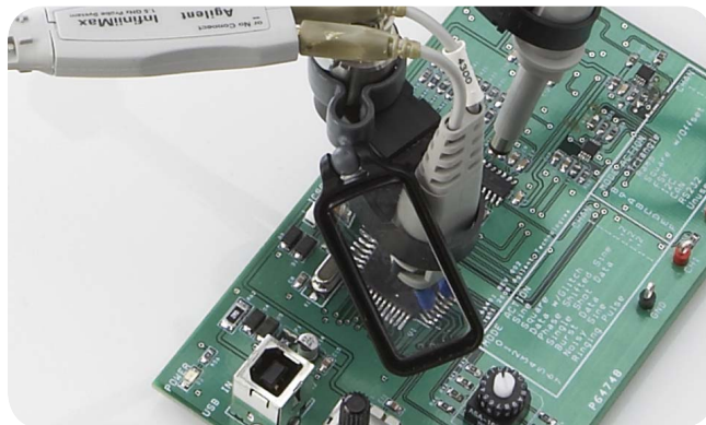
Figure 3. See a close-up view of the probing contact through the included 3X magnifying glass
